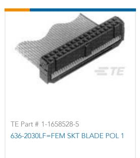
Ribbon Cable Connectors, Wire-to-Wire, 20 Position, 2.54 mm [.1 in] Centerline, Vertical, Through Hole - Solder, Insulation Displacement (IDC), 2 Row
